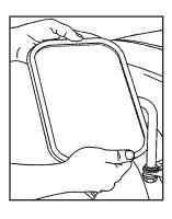
Turn the mirror head so that it swings further outboard and adjust the mirror surface as needed.
